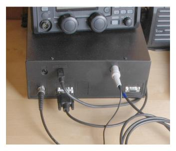
The second plug, the 8 PIN DIN plug (with blue label) goes into the ACC socket at the rear side of your M802. The Navilock GPS receiver is now getting his DC from the radio unit when you switch the radio on. When the GPS receiver has a fix, a steady green light will appear. Position and time in UTC will be shown on the display of the M802 control unit.
